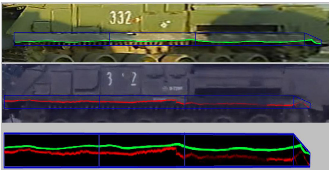
"Fingerprint" comparison between Buk 332 and Buk 3x2
