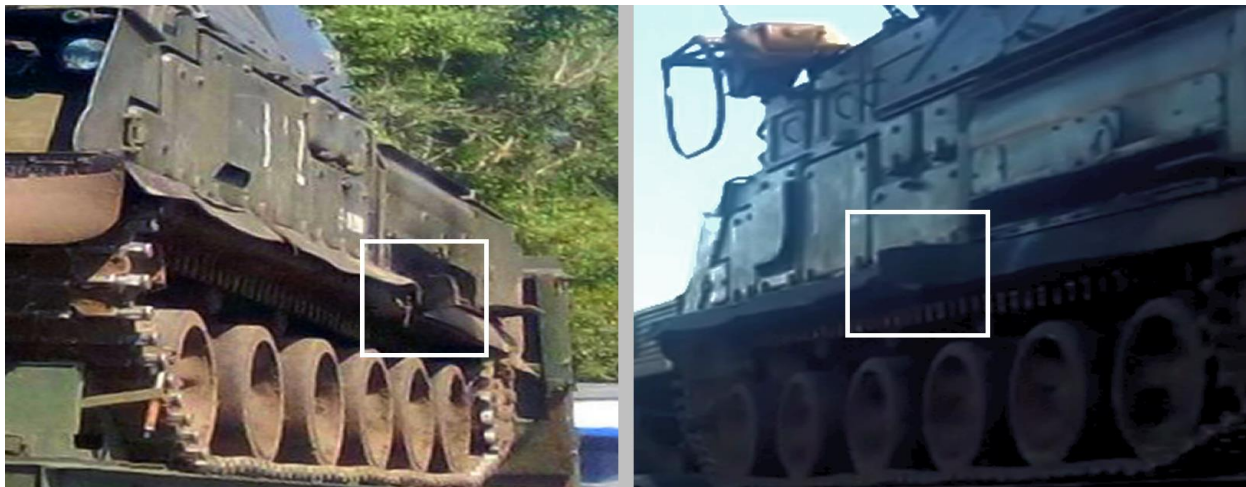
Figure 25: Damage to the side skirt visible on Buk 3x2
