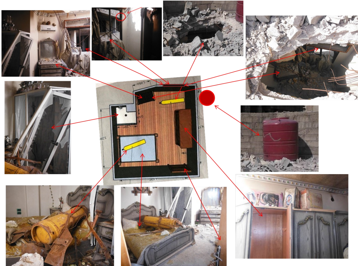
Figure 13: LAYOUT (TO SCALE) OF LOCATION 4 ("CYLINDER ON THE BED") SHOWING THE LIKELY IMPACT POINT OF THE ALLEGED WEAPON ON ENTERING THE APARTMENT AND THE FINAL RESTING PLACE ON THE BED.
